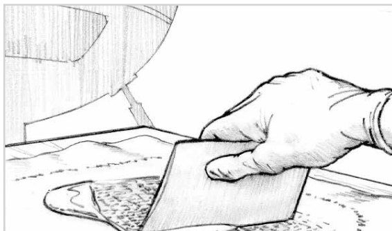
Figure 12-14 Wet out each piece of cloth with unthickened epoxy and squeegee into place.
