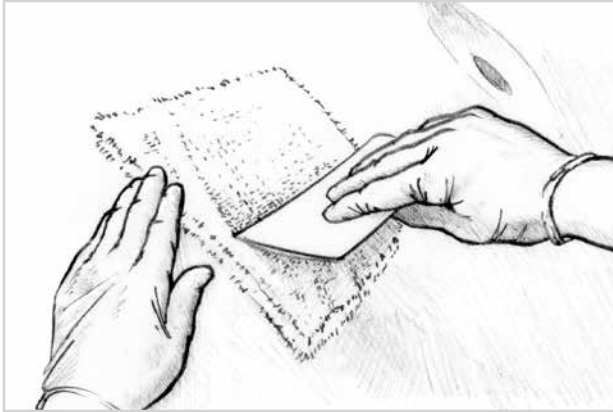
Figure 4-3 Smooth the wet-out fabric against the waxed panel to laminate a backer that matches the panel contour.
