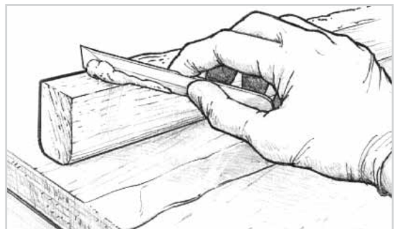
Figure 16-9 Apply enough thickened epoxy to one of the bonding surfaces so that a small amount will squeeze out of the joint when clamped with moderate pressure.
