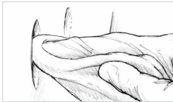
Figure 12-2 Wipe the cavity clean with alcohol and repeat until the laminate is dry to the touch.
