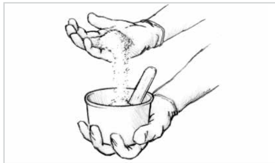
Figure 16-7 Blend in small handfuls or scoops of the appropriate filler until the desired consistency is reached.
