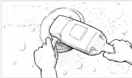
Figure 10-2 Use an electric polisher with an 8" foam sanding pad to open blister cavities or remove gelcoat.
