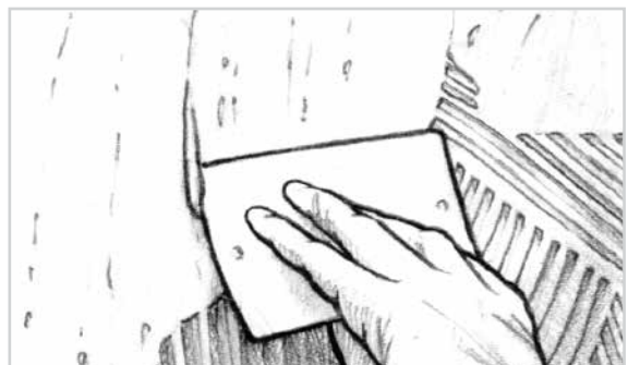
Figure 14-8 Trowel a second layer of fairing compound over the surface to fill the grooves after the ridges have been sanded fair.
